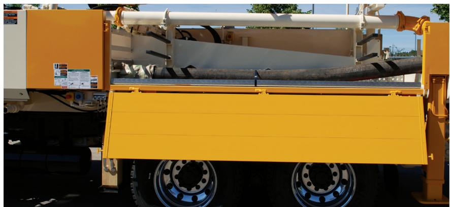
*Fold down sideboards store extra pipe and clamps for line pours and add to the pump's high utilization for owner operators, contractors or pumping fleets. Compact size makes this pump more maneuverable than larger pumps for better job site access.*
