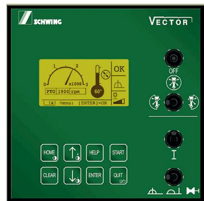
*Patented **Vector Controls** allow two-way communication between pump and operator. Critical real-time operating data is displayed at the remote box and stored in the controller for easy retrieval.*
