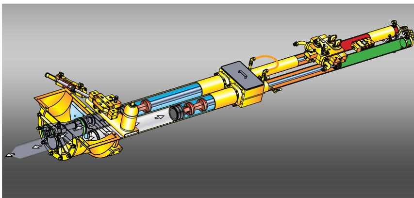
*This open loop all-hydraulic concrete pump sets the standard for fuel-efficiency, reliability and performance. Easily switch the hydraulics from the rod side to the piston side for higher pressure applications. **Rock Valve™** is designed to pump the harshest mixes and provide the lowest per yard operating costs.*
